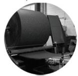
STEP FIVE: The underlayment is fusion bonded to a myriad of wear layers.
